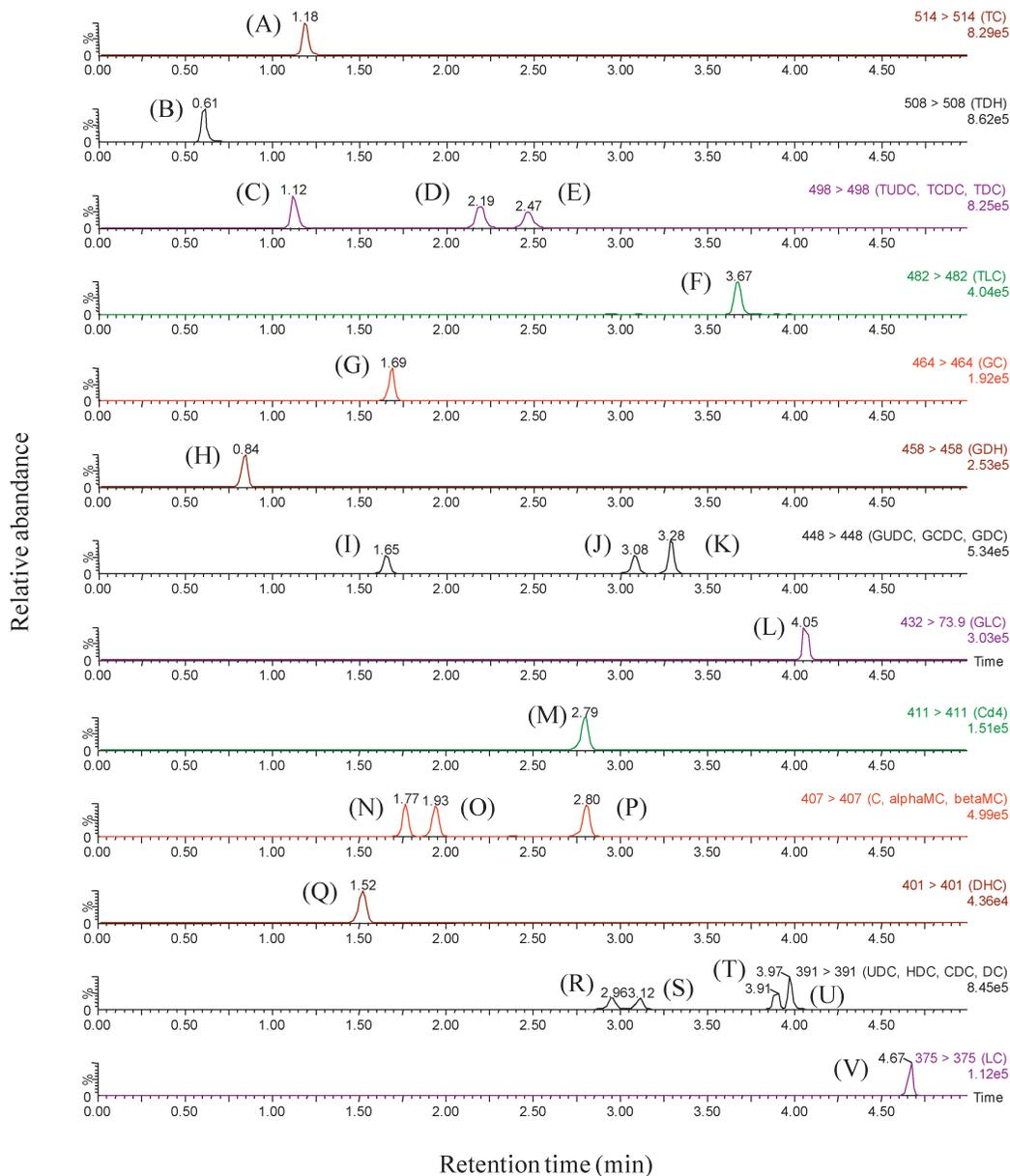
**Fig. 2** Multiple reaction monitoring (MRM) chromatograms for (A) TC, (B) TDHC, (C) TUDC, (D) TCDC, (E) TDC, (F) TLC, (G) GC, (H) GDHC, (I) GUDC, (J) GCDC, (K) GDC, (L) GLC, (M) IS, (N)  $\alpha$ -MC, (O)  $\beta$ -MC, (P) C, (Q) DHC, (R) UDC, (S) HDC, (T) CDC, (U) DC, and (V) LC, obtained by UPLC-MS-MS.
