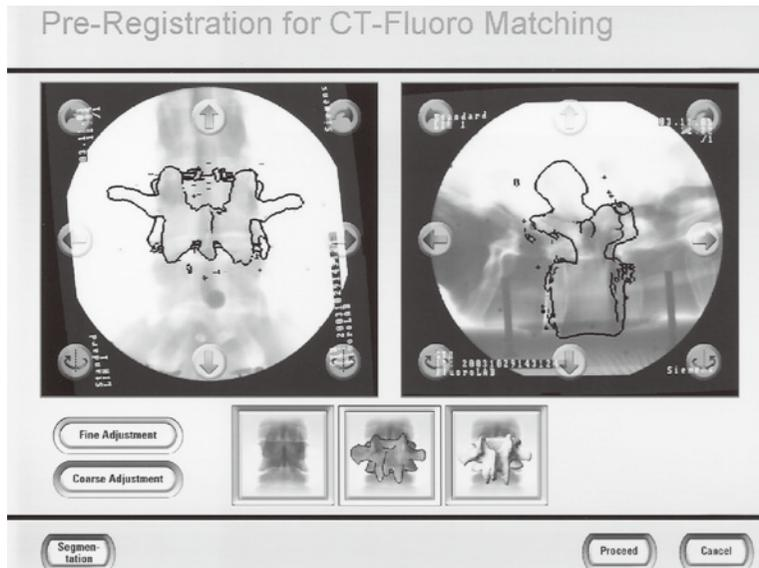
**Fig. 3** Pre-registration for CT-fluoro matching. Segmented vertebra is positioned over AP and lateral fluoroscopic images. Matching segmented vertebra as closely as possible to corresponding vertebra in fluoro image ensures best possible registration accuracy.
