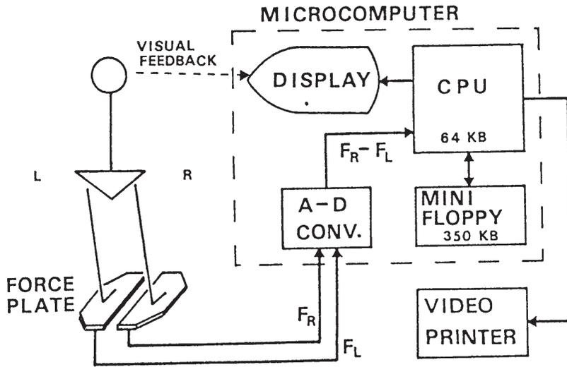
Fig. 1. Diagram of weight balance analyzer
