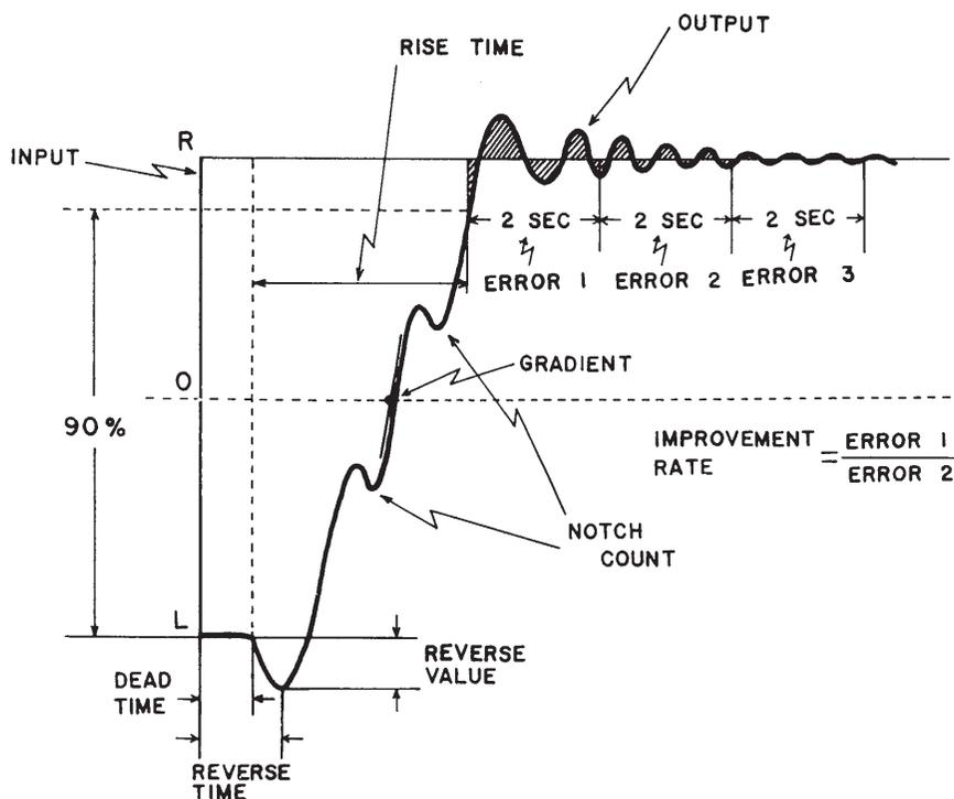
Fig. 3. Parameters of step response
