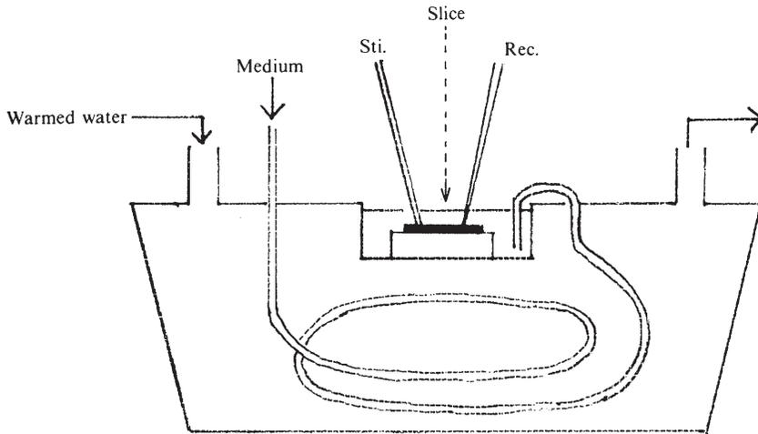
Fig. 2 Schematic drawing of the observation chamber.
