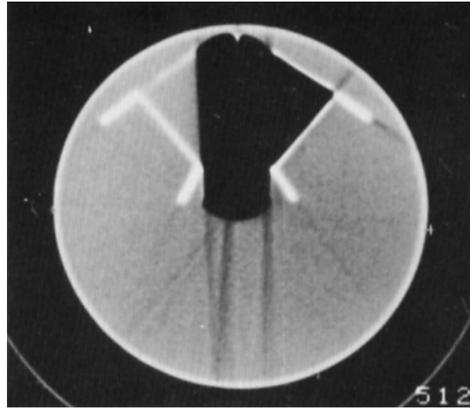
Fig. 2B. CT images of the phantom taken by Scanner I in Experiment 2. Wall B disappeared.
