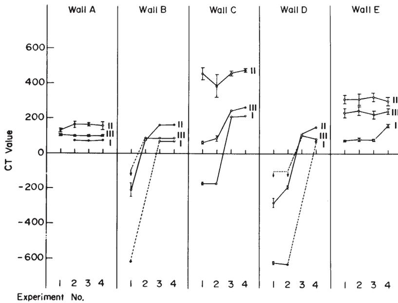
Fig. 8. The average peak X-axis CT values of Walls A to E at the level of the phantom corresponding to the posterior portion of the maxillary sinuses obtained by the three CT scanners.
