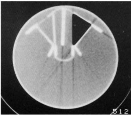
Fig. 2C. CT image of the phantom taken by Scanner I in Experiment 3. Wall D disappeared.
