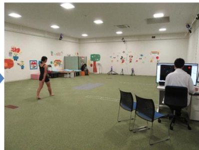
② 8 optical cameras capture motion during walking.
