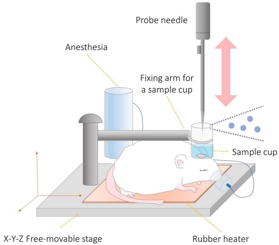
Fig. 3 Schematic image of a free-movable stage.
