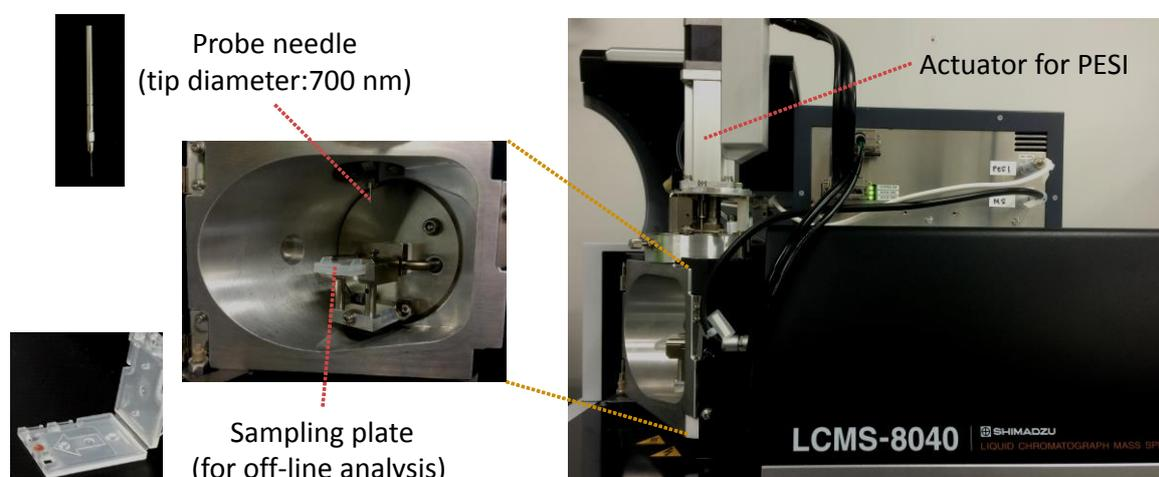
Fig. 1 Photograph of the probe electrospray ionization source combined with a triple quadrupole tandem mass spectrometer.
