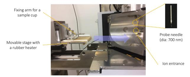
Fig. 2 Photograph of a newly-developed in vivo real-time monitoring system.
