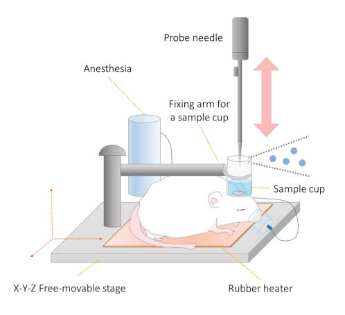
Fig. 3 Schematic image of a free-movable stage.
