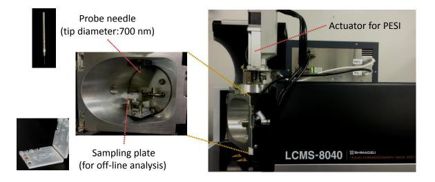
Fig. 1 Photograph of the probe electrospray ionization source combined with a triple quadrupole tandem mass spectrometer.
